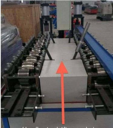
Handles to sheft gears between left & right roll forming machines
