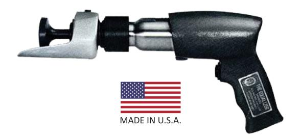
Here's the Pittsburgh Lock Seam Superior Air Hammer that can cut your finishing time up to 80%. They can be used to fold over or "seam" metal to 22 gauge and lighter on general fabricating, run Pittsburgh Lock Seams on ductwork, tubes, doors, panels, etc. Operators require no special training or skill. The finished seam is neater and more uniform than seams hammered by hand. Fabricating plants using the adapters claim that one operator's production equals that of eight hand-hammering workmen.
