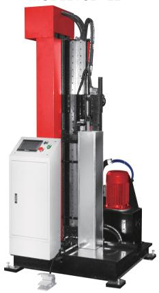
This machine can be used with DUCT AUTO LINE, TDF TRANSVERSE FLANGE DUCT MACHINE or TDC TRANSVERSE FLANGE DUCT MACHINE and PITTSBURGH LOCK MACHINE. The ideal duct connection includes united joint and right-angle side. The seam lock machine HFJ12 works out seam of high quality without help of other auxiliary connecting tool.
