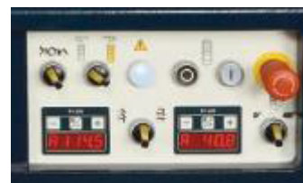
Powered spindle moulder unit positioning with digital display (in option for T55W)
