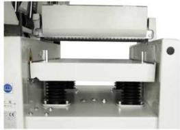
LONG LASTING STABILITY AND PRECISION: the thicknessing table lifts on 4 spindles with dust protected trapezoidal threads
