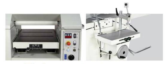
GREAT OPERATING COMFORT: powered height adjustment of the thicknessing table with display. For demanding machinings, it is available the thicknessing table with two removable idle rollers (option)
