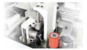
Absolute precision provided by the end cutting unit, powered by an independent motor that cuts off precisely at 90°, with a blade, any edge excess. Using the numeric readout the blade projection can be adjusted according to the thickness of the edge to be applied.
