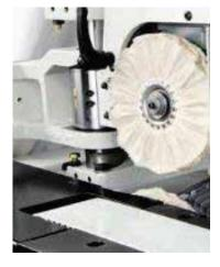
Superb finishing quality thanks to the edge scraping unit (optional) with a very strong structure guaranteed in any working condition. Precision positioning is assured by pad copiers. With a practical device for unit exclusion when it is not in use.
