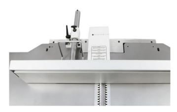
• TOTAL SAFETY AND CONTROL, high rigidity fence with a smooth movement due to the central locking on round bar
