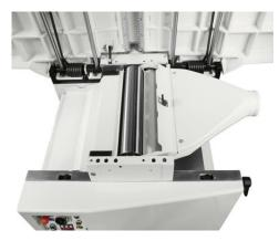
· OPTIMAL PLANNING WITH MINIMUM EFFORT, with the 120 mm spindle diameter and 4 knives
